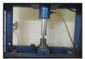
Figure (1) Compaction press used in the research.
