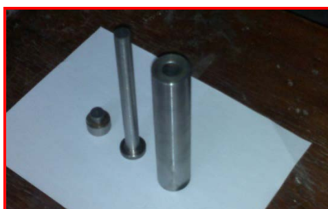
Figure (4): Cylindrical steel die with (15 mm) diameter.
