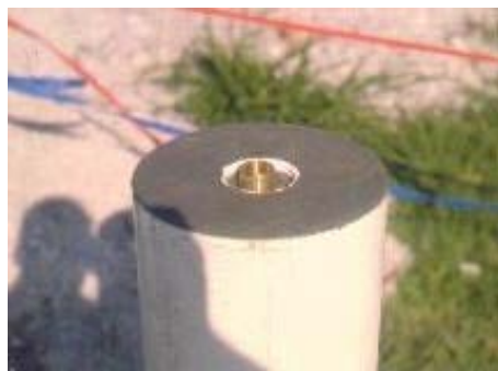
Figure (3) Typical pillar and details used for horizontal control. [10].
