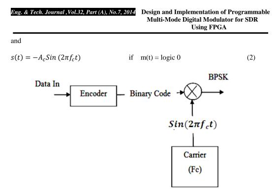
Figure (2): Bock diagram of BPSK modulator design
