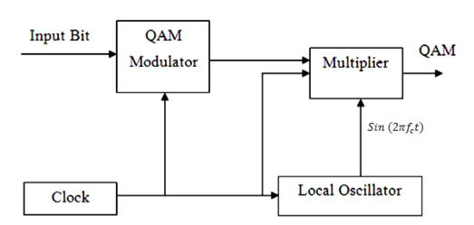
Figure (1) Block Diagram of QAM Modulator
