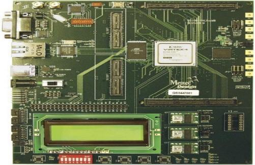
Figure (7): Virtex-4 System Board [13]
