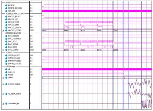
Figure (6): HDL simulation result of QAM Netlist
