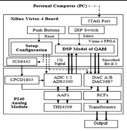
Figure (9): Hardware Implementation of FPGA and P240.
