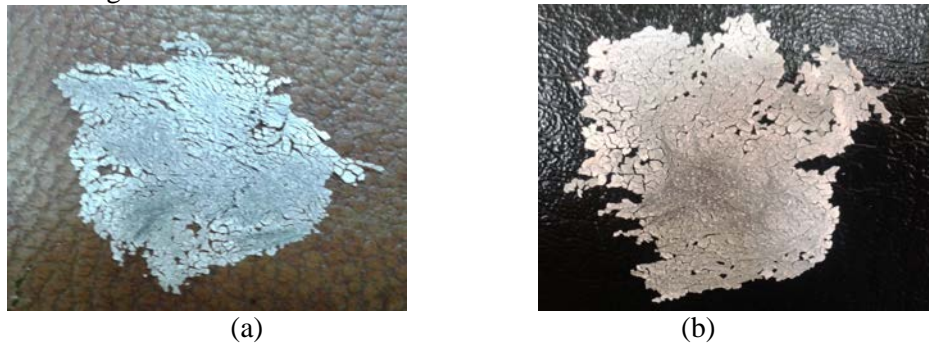
Figure (2) Coated carbon fibers – with adding HAP. (a) Untreated carbon fibers. (b) Treated carbon fibers.
