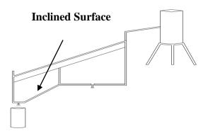
Fig. (2): The Designed Still (Front View).
