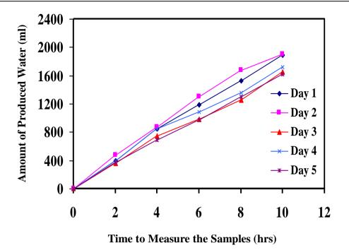
Fig. (6): The Amounts of Produced Well Water (ml) during Five Days.
