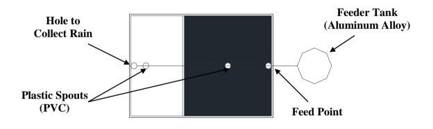
Fig. (4): The Designed Still (Top View).
