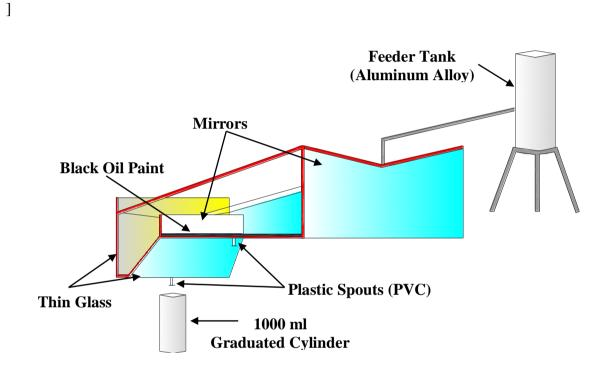
Fig. (1): The Designed Still (3D View).
