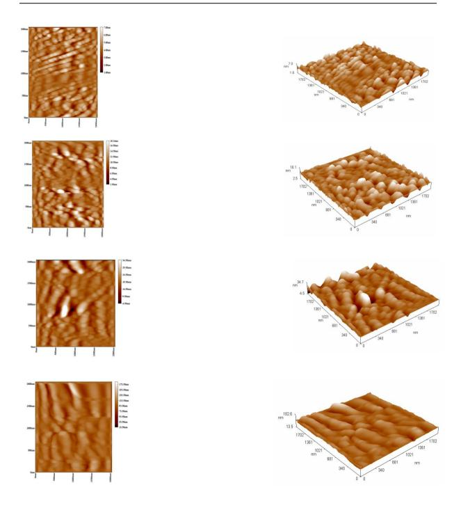
**Fig (2):** 2D and 3D AFM images for Mg AZ31 Alloy (a) polished Surface (b) 10min.Anodizing (c) 20 min. Anodizing (d) 30 min. Anodizing
