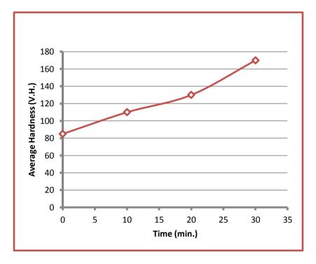
Fig (6): Relation between anodizing time and microhardness of coating layers
