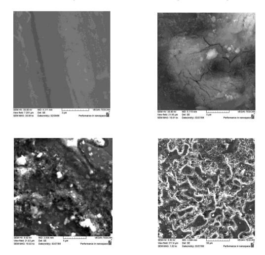
**Fig. (4):** SEM morphology of the anodic surface: (a) polished Surface (b) 10 min. Anodizing (c) 20min.Anodizing (d) 30min.Anodizing
