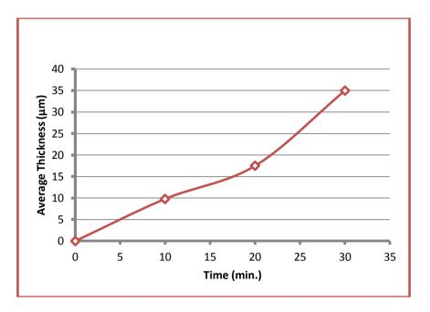
Fig (5): Variation of coating thickness with anodizing time
