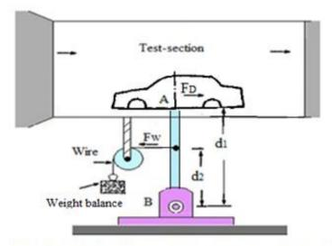
Fig.(5): Installation Details of the Single Component Balance Device.
