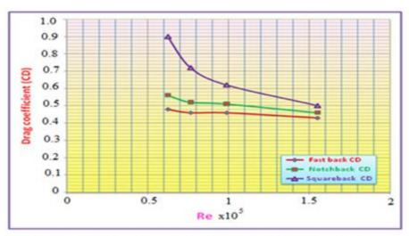
Fig.(12): Drag Coefficient (CD) Variation with Reynolds Number for the Different Three Configurations.
