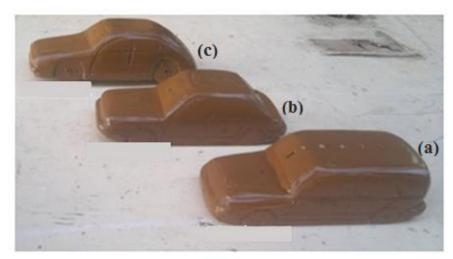
Fig.(3): Experimental Models (a)Squareback, (b)Notchback and (c) Fastback.
