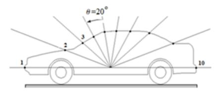
Fig.(6): Tested Model with Pressure Tapping.
