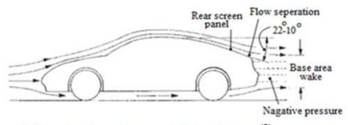
Fig.(1): Design of Road Vehicles Rear End Configuration<sup>(3)</sup>.
