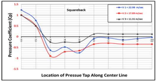
Fig.(7): Variation of Pressure Coefficient (Cp) along the Center Line of Squareback Configuration and for Different Three Velocities.
