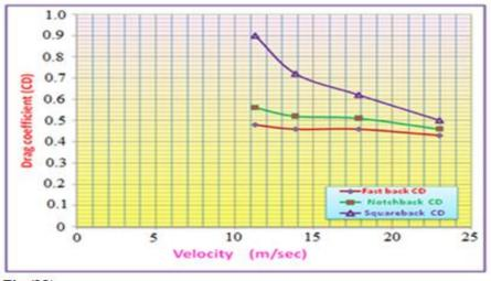
Fig.(11): Drag Coefficient (CD) Variation with the Free stream Velocity for the Different configurations.
