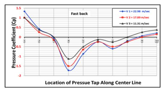
Fig.(9): Variation of Pressure Coefficient (Cp) along the Center Line of Fastback Configuration and for Three Velocities.
