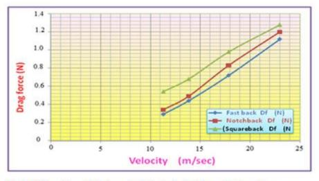
Fig.(10): Drag Force Variation with Velocity for the Three Configurations.
