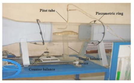
Fig.(4): Wind-tunnel Test Section with Single Component Balance for Drag Force Measurements.
