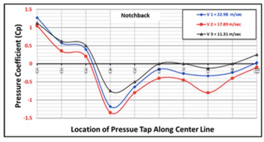
Fig.(8): Variation of Pressure Coefficient (Cp) along the Center Line of Notchback Configuration and for Different Three Velocities.
