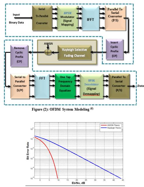
Figure (3-a): The BER performance conventional OFDM over Two channels scenarios.
