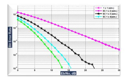
Figure (7): BER of SC with different number of receive antennas.
