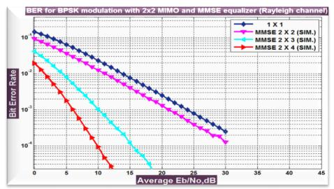
Figure (13): BER performance of MMSE with  $M_T = 2$  and  $M_R = 2, 3, and 4$
