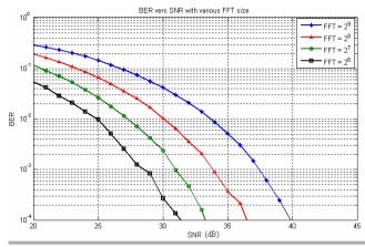
Figure (3-b): OFDM performance under various FFT size
