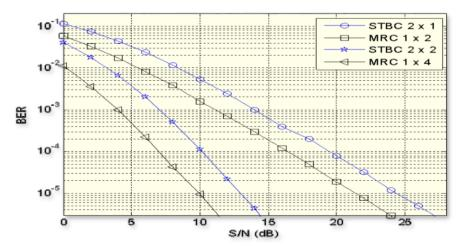
Figure (16): BER performance comparison between STBC and MRC methods
