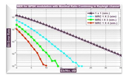
Figure (9): BER of MRC with different number of receive antennas
