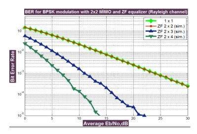
Figure (12): BER performance of ZF with  $M_T = 2$  and  $M_R = 2$ , 3, and 4
