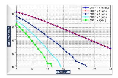
Figure (8): BER of EGC with different number of receive antennas
