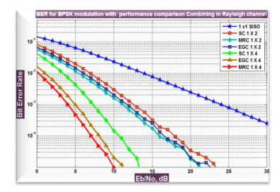
Figure (11): BER performance comparison of SC, EGC and MRC with different number of receive antennas
