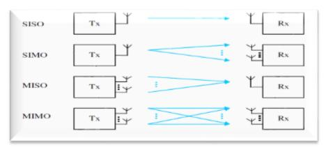
Figure (1) Types of antenna (SISO, SIMO, MISO, and MIMO)
