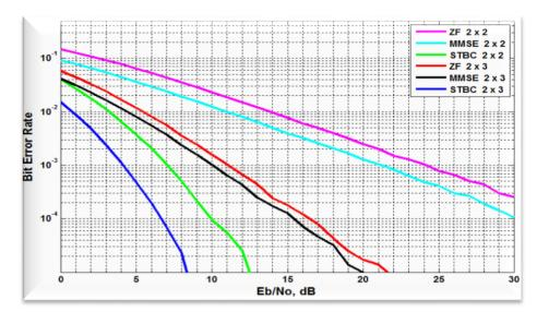
Figure (17): BER performance comparison between ZF,MMSE and STBC methods
