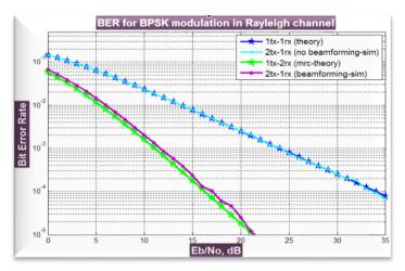
Figure (10): BER performance comparison between MRC and MRT
