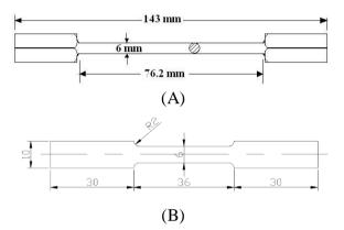
Fig. (1): Testing specimens of Brass C<sub>38500</sub>,(A) Torsion specimen,(B) Tensile specimen.
