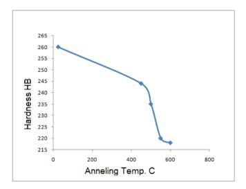
Fig (3): the relationship between annealed temperature and hardness.
