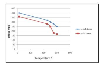
Fig (5): the relationship between stress and annealing temperature.
