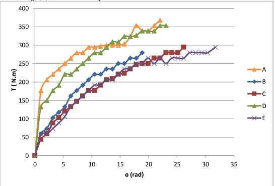
Fig. (7): the relationship between torque and twist angle.
