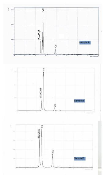
Fig (4): phases analysis graphs for specimen for A, B and E.
