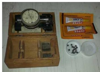
ELE extensometer and demec discs
