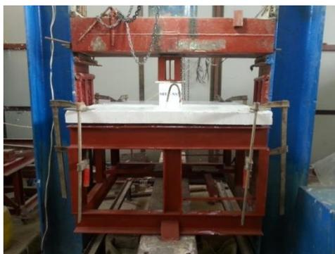
**Figure (6):** Apparatus of the testing of slab-column models
