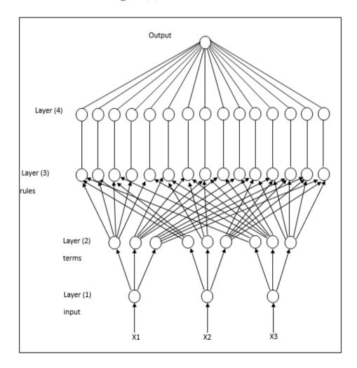
Figure (10): Adaptive neuro-fuzzy inference system architecture.
