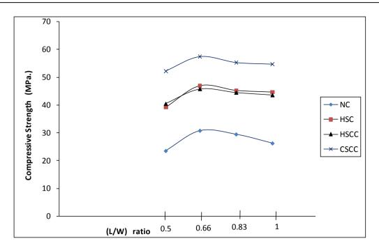
Figure (1): Relation between (L/W) ratio and compressive strength of (150\*150\*150) mm cubes.
