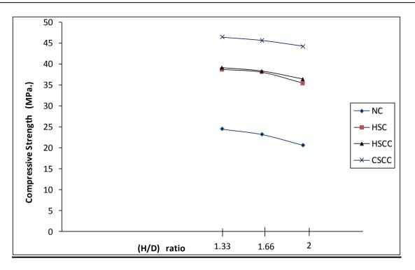
**Figure (3):** Relation between (H/D) ratio and compressive strength of (150\*300) mm cylinders.
