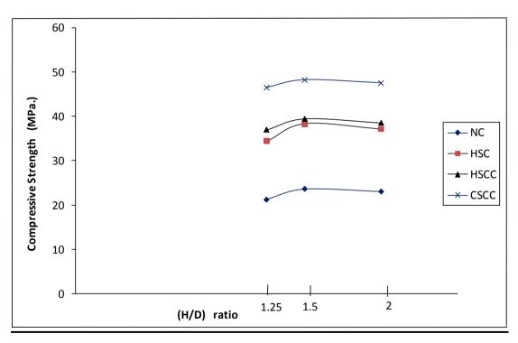
Figure (4): Relation between (H/D) ratio and compressive strength of (100\*200)mm cylinders.
