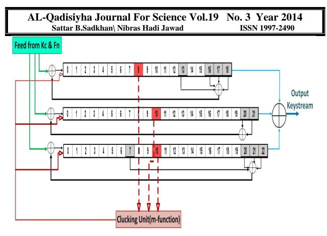
Figure (1) structure of A5/1 generator
