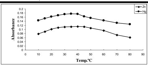
Fig.(7 )Effect of the temperature on the absorbance for (6- MBTADI)- M(II) complexes formed with Zn (II) and Hg (II) ). Conditions : Zn(II) = 15  $\mu$ g mL<sup>-1</sup>, 3 ml of (6- MBTADI) =1.75x10<sup>-4</sup> M .and Hg(II) = 6  $\mu$ g mL<sup>-1</sup>, 1.5 ml of (6- MBTADI) =1.75x10<sup>-4</sup> M
