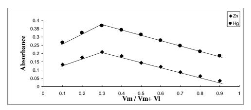
Fig.10 Continuous variation method for Zn(II)-complex at pH=6 and Hg(II)complex at pH=5
