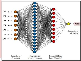
Fig. 22: Configuration of Neural Network 7-17-9-1.
