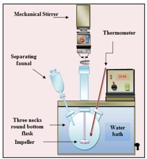
Fig. 2-a: The reaction system
