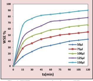
Fig. 6: WSE vs. separation time at different doses of BCO.
