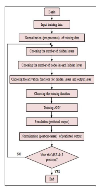
Fig. 24: The Structure of the Neural Network Program
