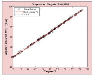
Fig. 20: Testing Regression of the Proposed Neural Network.
