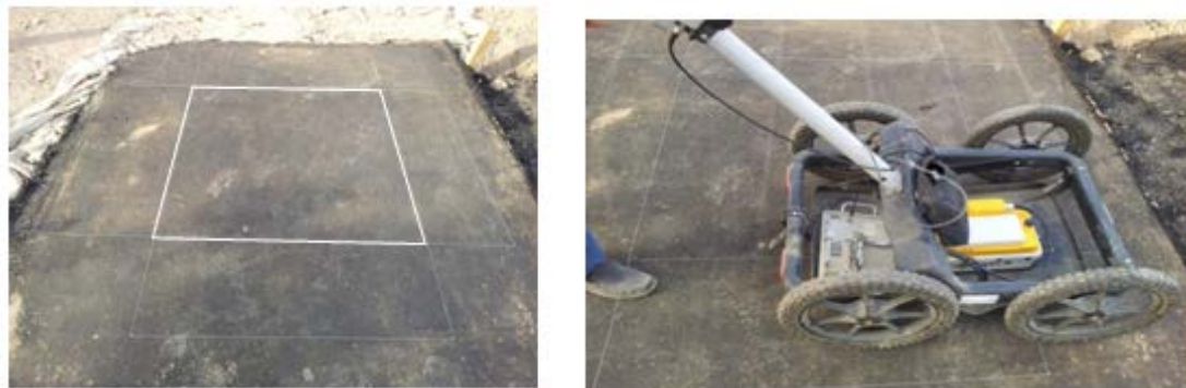
Figure (5) Inspecting the in-situ simulation model by GPR.
