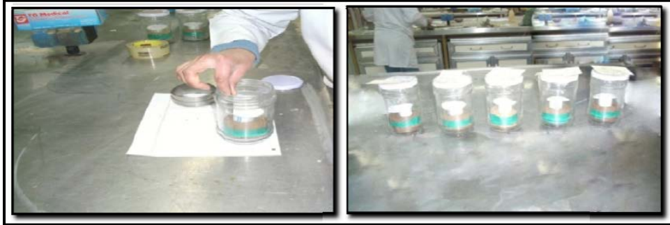
Figure (4) Steps of the total suction measurements (after Mohsin, 2012).
