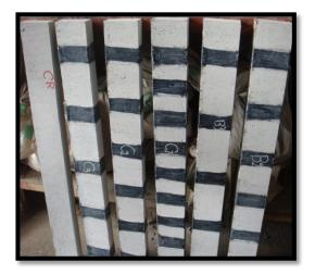
Plate (2) Beams Strengthened with CFRP.
