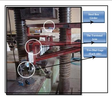
Plate (3) Testing Setup.
