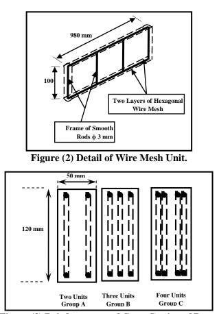
Figure (3) Reinforcement of Cross Section of Beams.
