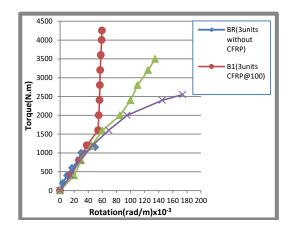
Figure (10) Torque-Rotation Relationships for Group B(Effect of Spacing of CFRP Strips).
