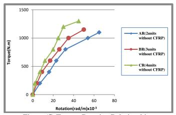
Figure (5) Torque-Rotation Relationships (Effect Number of Units).
