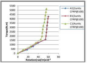
Figure (8) Torque-Rotation Relationships (Effect Number of Units).
