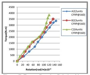
Figure (7) Torque-Rotation Relationships (Effect Number of Units).
