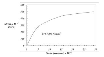
Figure(1) Stress–Strain Curve of the Wire Mesh(12) 2-1-6 Mold.
