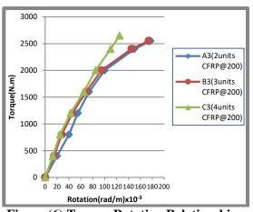
Figure (6) Torque-Rotation Relationships (Effect Number of Units).
