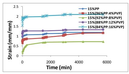
Figure (13) Creep behavior of [84%LLDPE:15%((100-X)%PP:X%PVP):1%B.P] as a function of PVP content in the composites.
