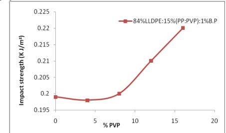
Figure (10) Impact strength of [84%LLDPE:15%((100-X)%PP:%XPVP):1%B.P] as a function PVP content in the composites.
