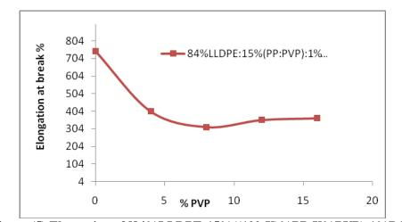
Figure (5) Elongation of [84%LLDPE:15%((100-X)%PP:X%PVP):1%B.P] as a function of PVP content in the composites.
