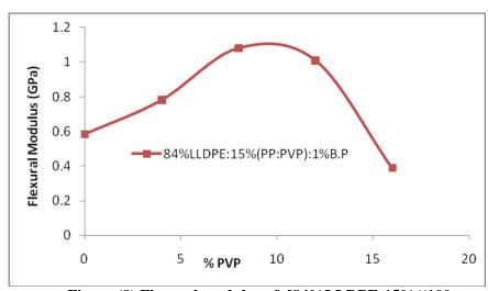
Figure (9) Flexural modulus of [84%LLDPE:15%((100-X)%PP:X%PVP):1%B.P] as a function of PVP content in the composites.
