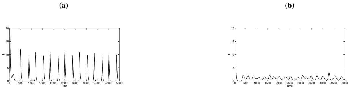
Fig (14) : Temporal variation of intensity of quantum dash semiconductor laser for various combination of ( \eta , g , f(\text{Hz}) , R , J_b and J_a )
