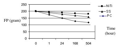
Figure (1): Force - time diagram of PC, NiTi CCS and SS CCS in dry condition.
