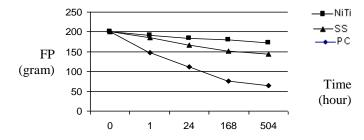
Figure (2): Force - time diagram of PC, NiTi CCS and SS CCS in artificial saliva of normal pH.
