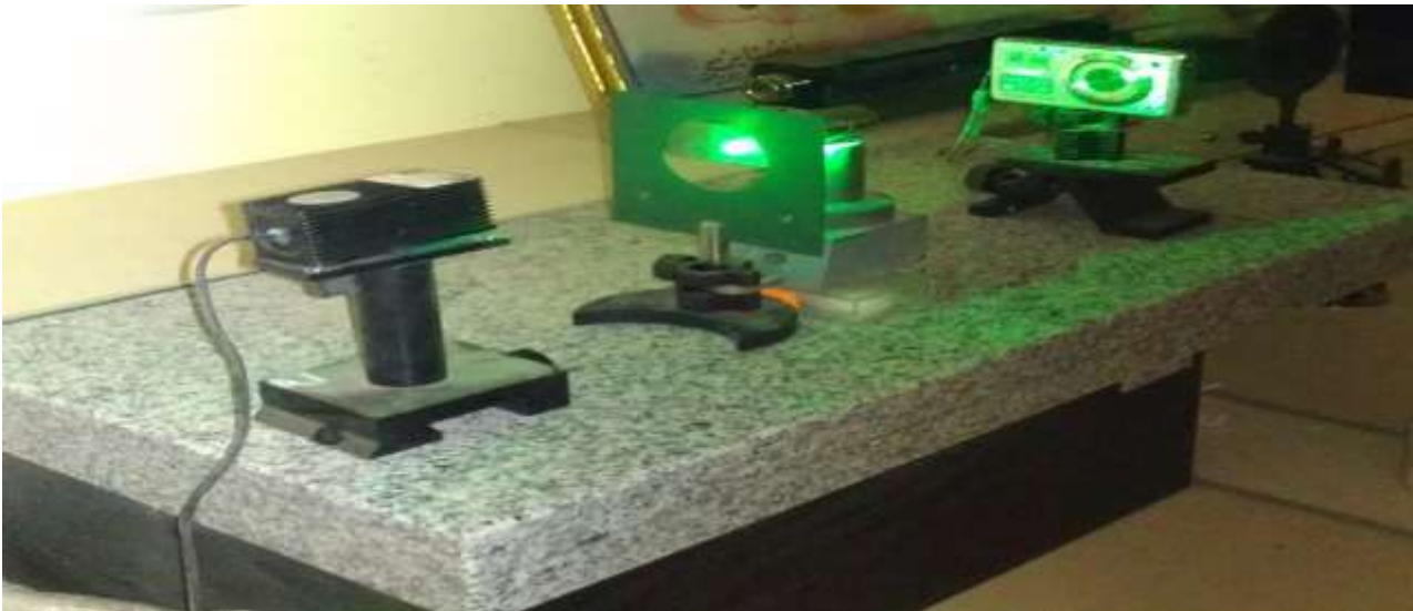
Figure 5 Photograph for Setup of The DHM.(Karbala University ,College Of Science )
