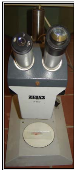
Figure (3): Stereoscopic microscope at 40X magnification
