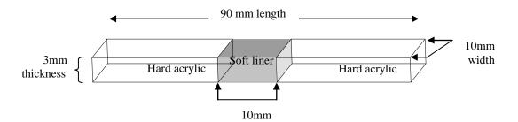
Figure (1): Diagram of tensile test specimens.
