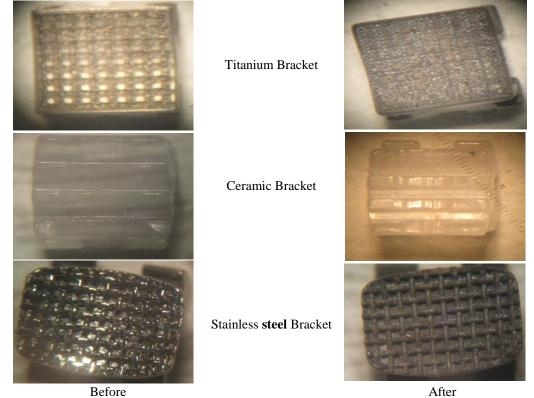
Figure (1) Different orthodontic bracket base before and after etching under stereo microscope
