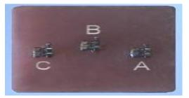
Figure (1): Acrylic Block on which a Standard Stainless steel Brackets Fixed.
