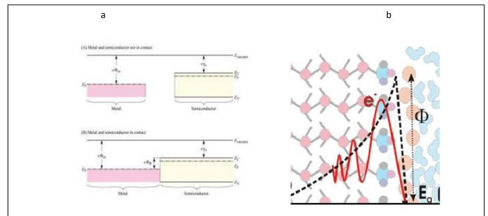
*Figure (1): Schematic illustration of (a) model potential of electron transfer at band probability at the metal/semiconductor[11], and (b) tunneling process[12].*
