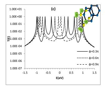
Fig.(3): The transmission probability as function of the system energy with presence magnetic flux at  $\phi = 0.3\pi$ ,  $0.6\pi$ ,  $0.9\pi$  for three configurations are para in (a), meta in (b) and ortho in (c). The parameters are  $E_{B1} = E_{B2} = E_{B3} = E_{B4} = E_{B5} = E_{B6} = 0$ ,  $V^{DB} = V^{AB} = -0.3eV$ ,  $V^{BB} = -0.5eV$ ,  $V^{AR} = -3eV$ ,  $\beta_R = -3eV$ .
