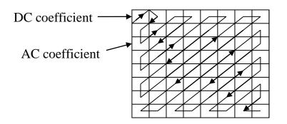
Figure (5): Properties of DCT Coefficients of 8x8 Blocks with Zigzag Pattern
