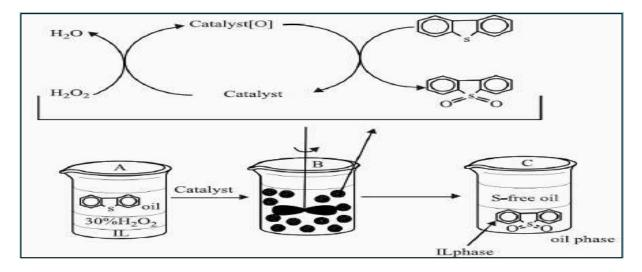
Scheme 1. Mechanismof the oxidation of dibenzothiophene.
