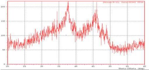
Figure 1X-ray diffraction patterns of the Cat- B 1 Ni : Co :  $\gamma$ -Al<sub>2</sub>O<sub>3</sub> (15: 5 : 80)
