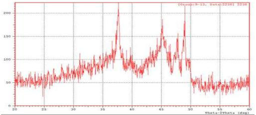
Figure 2X-ray diffraction patterns of the Cat- B 2 Ni : Co :  $\gamma$ -Al<sub>2</sub>O<sub>3</sub> (16: 4 : 80)
