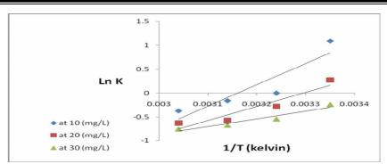
Figure (3): The relationship between LnK<sub>d</sub> and 1/T of activated carbon at different concentrations
