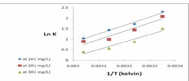
Figure (2): The relationship between LnK<sub>d</sub> and 1/T of clay at different concentrations
