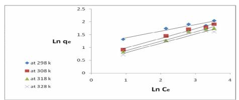
Figures (5): The relationship between Ln qe versus Ln Ceq at various temperatures on activated carbon
