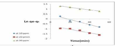
Figure (9): Pseudo first order rate plot for Cu<sup>+2</sup> ions adsorption by the clay at various initial concentrations
