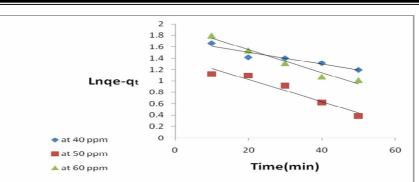
Figure (10): Pseudo first order rate plot for Cu<sup>+2</sup> ions adsorption by the clay at various initial concentrations
