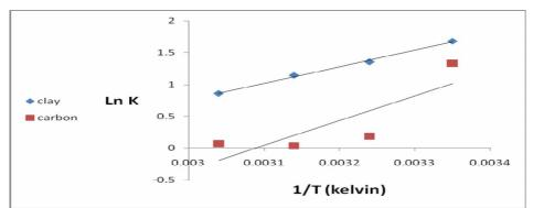
Figure (4): The relationship between Ln Kd and 1\T of clay and activated carbon by using Freundlich constant
