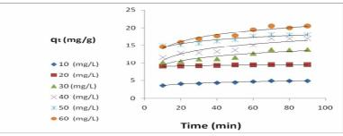
Figure 1: Variation of adsorption capacity of clay with time
