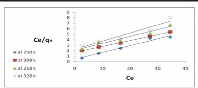
Figures (7): The relationship between Ceq/qe versus Ceq at various temperatures on activated carbon
