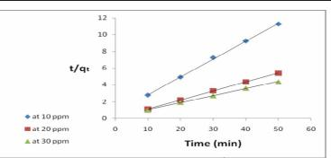
Figure (11): Pseudo second order rate plot for Cu<sup>+2</sup> ions adsorption by the clay at various initial concentrations
