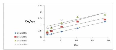
Figures (8): The relationship between Ceq/qe versus Ceq at various temperatures on clay
