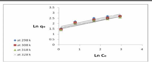
Figures (6): The relationship between Ln qe versus Ln Ceq at various temperatures on clay
