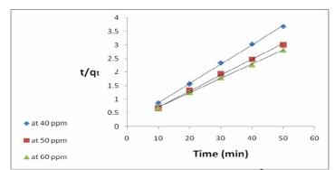
Figure (12): Pseudo second order rate plot for Cu<sup>+2</sup> ions adsorption by the clay at various initial concentrations
