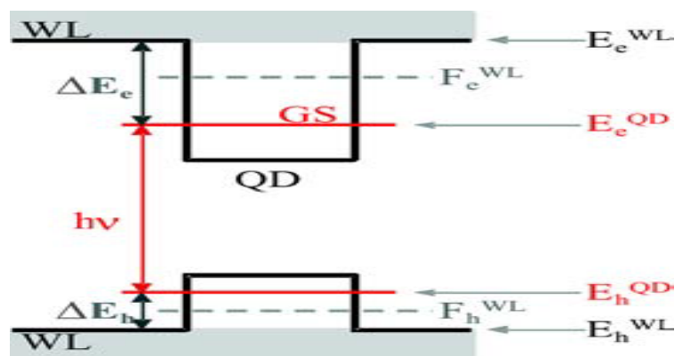
Figure 1: Energy diagram of the QD and WL system[6].
