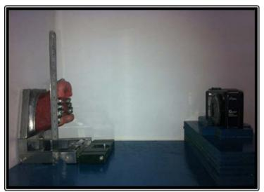
Figure (4): Wood table to which a metal base of typodont articulator and a ruler were attached to it.
