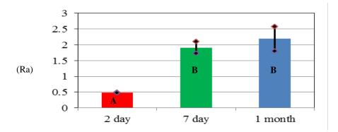
Means with the different letter are statistically significant different at p < 0.05Figure (15): Mean  $\pm$  SD and Duncan's multiple rang test of surface roughness for (Lacalute)
