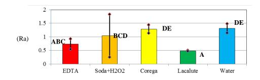
Means with the different letter are statistically significant different at p < 0.05 **Figure (9):** Mean ± SD and Duncan's multiple rang test of surface roughness for Comparison among time intervals. (2 Days)
