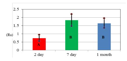
Means with the different letter are statistically significant different at p < 0.05 **Figure (13):** Mean ± SD and Duncan's multiple rang test of surface roughness for (Soda + H2O2)
