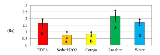
Means with the different letter are statistically significant different at p < 0.05Figure (11) :Mean  $\pm$  SD and Duncan's multiple rang test of surface roughness for Comparison among time intervals. (1 Month)
