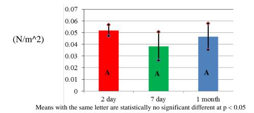
Figure (5): Mean ± SD and Duncan's multiple rang test of tensile strength for(Soda + H2O2)
