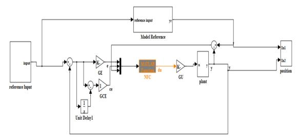
Figure (2): MATLAB/Simulink block diagram for Neuro-Fuzzy Model Reference Adaptive Control
