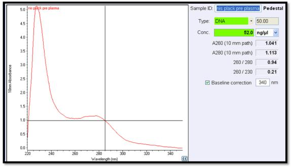
Figure (3): Measurement quantity of DNA (ng /  $\mu$ l) from pregnant females plasma using Nanodrop technique.
