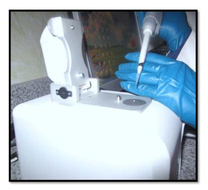
Figure(1): Showing measurement DNA quantity ng/ µlusing Nanodrop technique.
