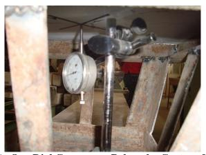
Fig. (4): One Dial Gauges are Below the Center of Slabs.
