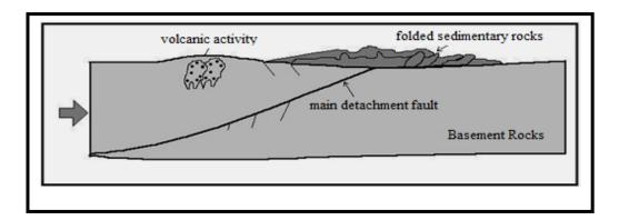
Fig. 13: Thin-Skinned Tectonics (From Kley et. al., 1999).
