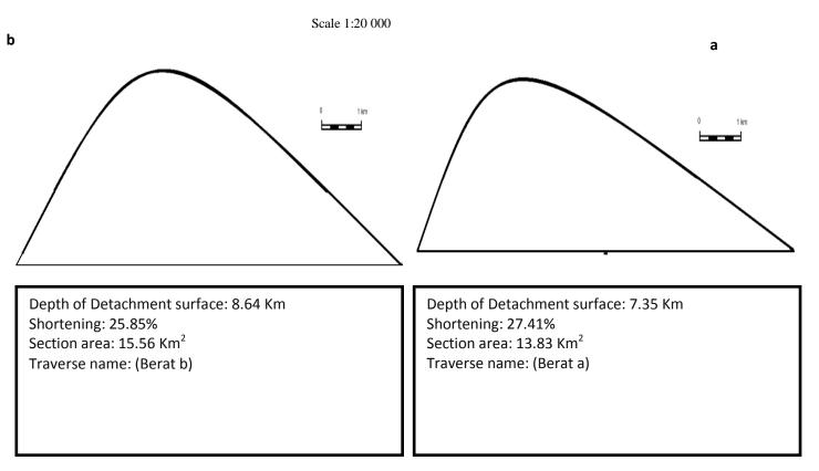
Fig. 6: a- Structural Profile for Traverse (1), b- Structural Profile for Traverse (2) of Berat Anticline.
