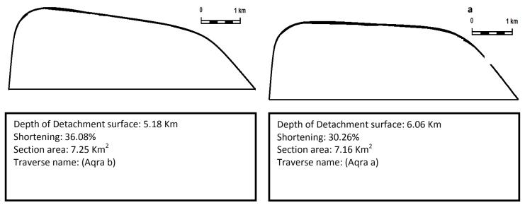
Fig. 5: a- Structural Profile for Traverse (1), b- Structural Profile for Traverse (2), of Aqra Anticline.
