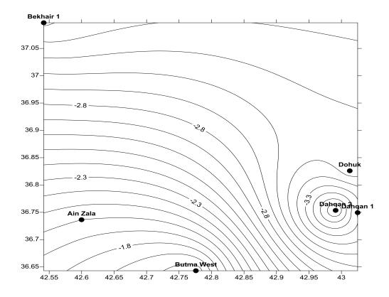
Fig. 16: a- The Contour Map for Depth of Detachment Surface Morphology for Thin–skinned.
