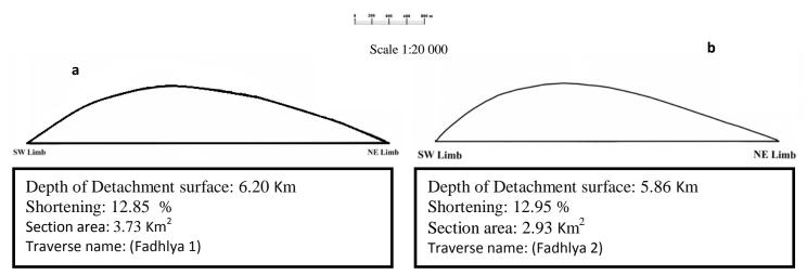
Fig. 8: a- Structural Profile for Traverse (1), b- Structural Profile for Traverse (2) of Fadhlya Anticline.
