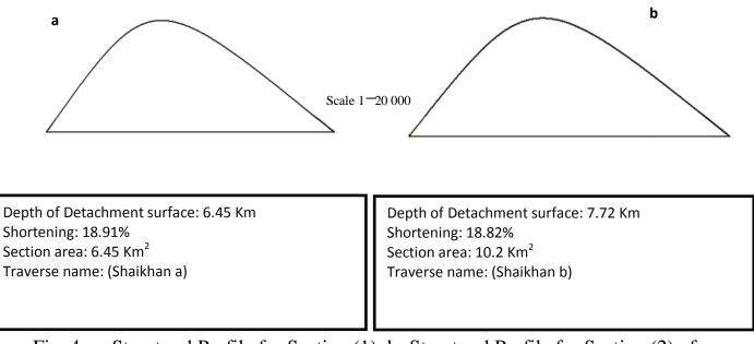
Fig. 4: a- Structural Profile for Section (1), b- Structural Profile for Section (2) of Shaikhan Anticline.
