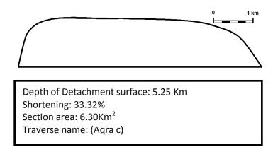
Fig. 5: c- Structural Profile for Traverse (3) of Aqra Anticline.
