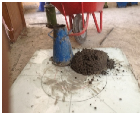
Figure(5) Slump test for mixture C5.
