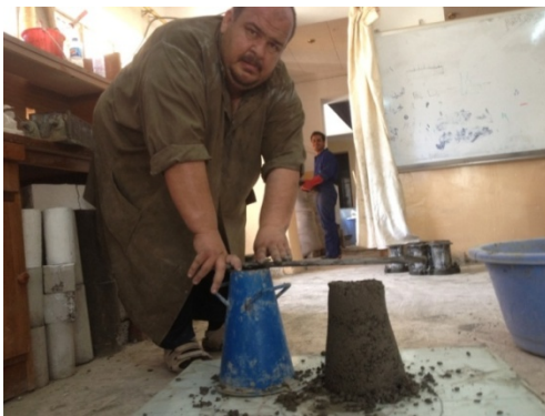
Figure(4) Slump test for mixture C1
