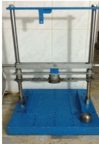
Figure (1) Drop weight machine.
