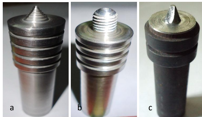
Figure (1) Tool designs used in FSW a) Mode 1, b) Mode 2, c) Mode 3.
