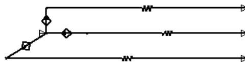
(b) Secondary load circuit represented by three stranded coil circuit elements, star connected with earthed common point, and a 3 phase resistive load.
