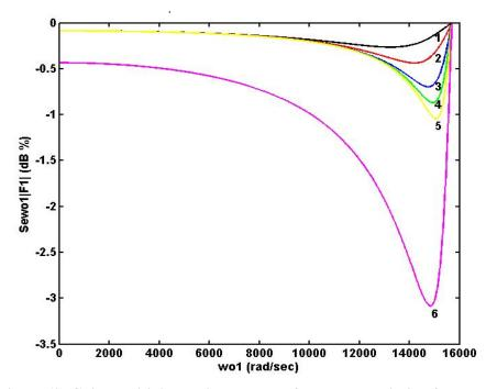
Figure (9) Gain sensitivity against angular frequency variation for the multiple-loop feedback bandpass filter for different values of quality factor in each stage.
