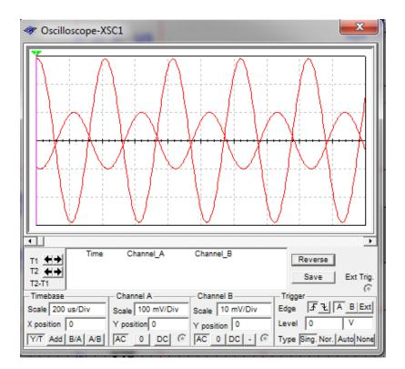
Figure (15) Input and output waveforms of the filter.
