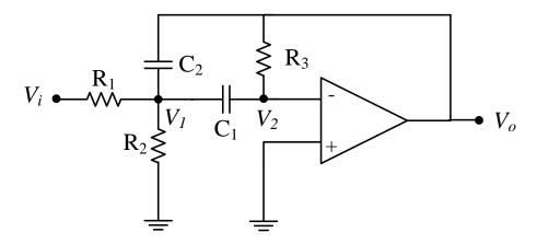
Figure (1) Multiple-loop feedback Second-order bandpass active filter network.
