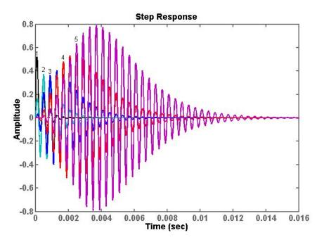
Figure (5) Step response for the multiple-loop feedback bandpass filter for different values of quality factor in each stage.
