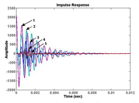
Figure (7) Impulse response for the multiple-loop feedback bandpass filter for different values of resonance frequency in each stage.
