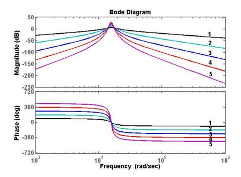
Figure ( 3) Bode plot for the of the tenth order multiple-loop feedback bandpass filter for different values of quality factor in each stage.
