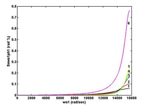
Figure (11) Phase sensitivity against angular frequency variation for the multiple-loop feedback bandpass filter for different values of quality factor in each stage.
