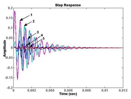
Figure (8) Step response for the multiple-loop feedback bandpass filter for different values of resonance frequency in each stage.
