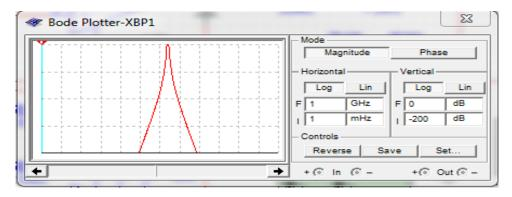
Figure (16) Multiple-loop bandpass filter response characteristic.
