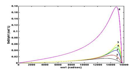
Figure (12) Phase sensitivity against quality factor variation for the multipleloop feedback bandpass filter for different values of quality factor in each stage.
