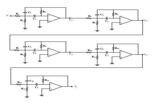
Figure (2) Multiple-loop feedback tenth order bandpass active filter network.
