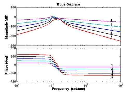
Figure (6) Frequency response of the tenth order multiple-loop feedback bandpass filter for different values of resonance frequency in each stage.
