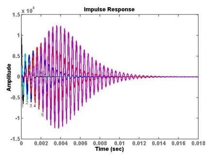
Figure (4) Impulse response for the multiple-loop feedback bandpass filter for different values of quality factor in each stage.
