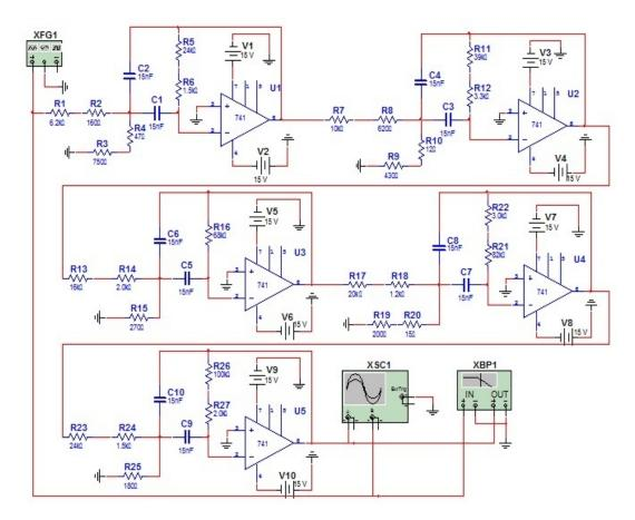
Figure (13) Multisim simulation of the multiple-loop feedback bandpass filter network.
