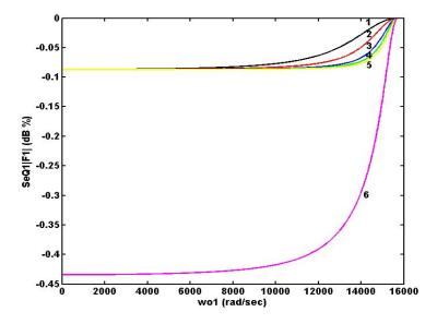
Figure (10) Gain sensitivity against quality factor variation for the multiple-loop feedback bandpass filter for different values of quality factor in each stage.
