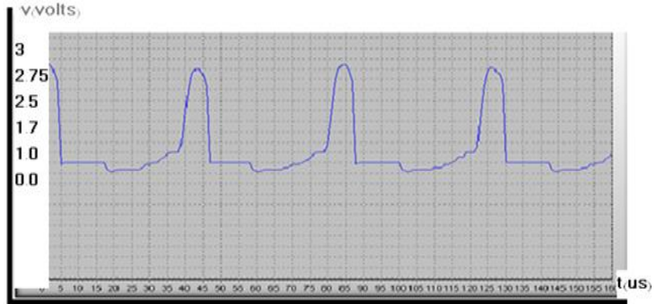
Figure (15a) O/p of pulse transformer to thyristor.
