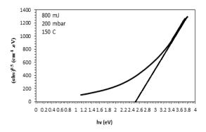
Fig (4) show the s a plot of  $(\alpha hv)1/2$  versus hv for energy gap value for Bi2O3 thin film
