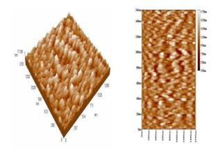
Fig (2) AFM image of Bi2O3 thin film prepared at optimum condition
