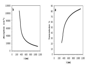
Fig (3) a) transmission of Bi<sub>2</sub>O<sub>3</sub> thin film b) absorption of Bi<sub>2</sub>O<sub>3</sub> thin film
