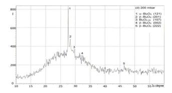
Fig (1) XRD of Bi2O3 prepared by pulse laser deposition at specific preparation condition
