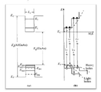
Fig.(2) (a) potential of quantum well and quantized levels. (b)density of states diagram and possible recombination [13].
