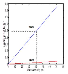
Fig.(4) The optical confinement factor as a function of the wire width for Al0.2Ga0.8As/ GaAs of MQWR structure.
