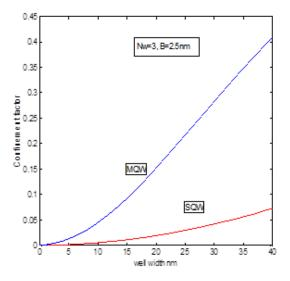
Fig.(3) The relation between confinement factor and well width of Al0.2Ga0.8As, x=0.2.
