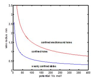
Fig.(8) Quasi-critical as a function of the band gap. Electrons and holes in quantum wires which are smaller than the quasi-critical radius are bound by the potential but are only weakly confined.
