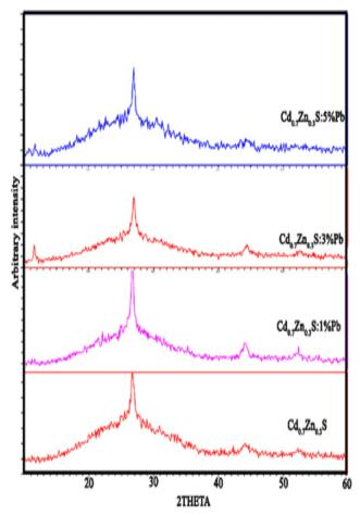
Fig. (1) The XRD pattern of thin films prepared
