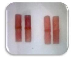
Figure (3) : Two Pairs of acrylic cylinders with Vertex and Molloplast–B lining materials placed in the space (2.5 mm thickness)
