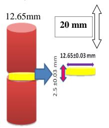
Figure (2): Pair of acrylic cylinders+ Rounded metal spacer
