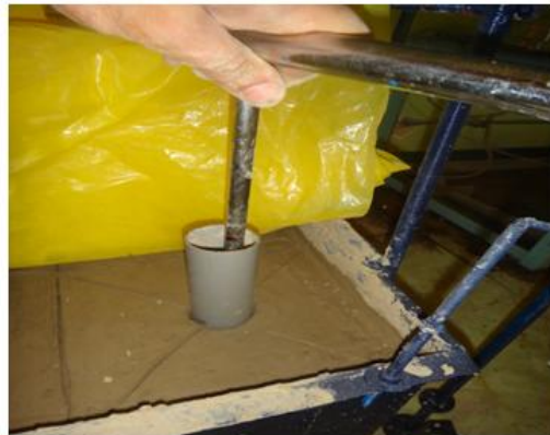
b): Make the hole of the stone column
