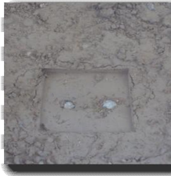
Plate (8) Two piles with raft after test.
