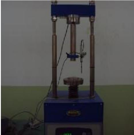
Plate (5) Load cell anted indicter
